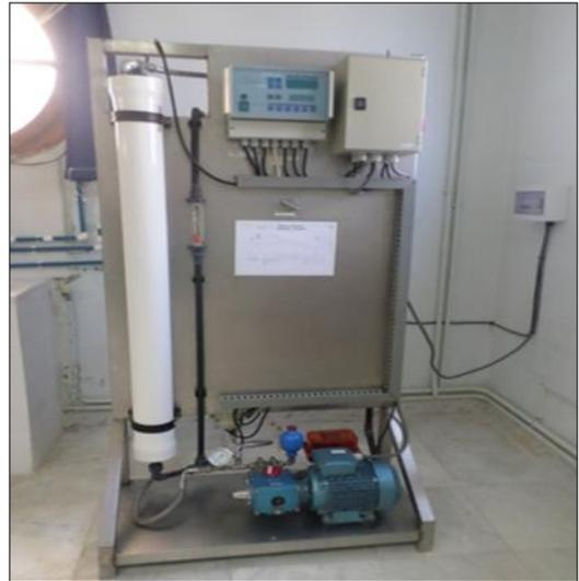
Fig1. Reverse Osmosis pilot installed in the DDEMS laboratory
