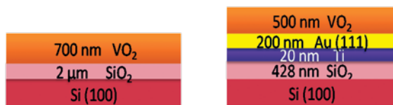
Fig. 1 : Schematic of the deposited VO _2 thin films.
