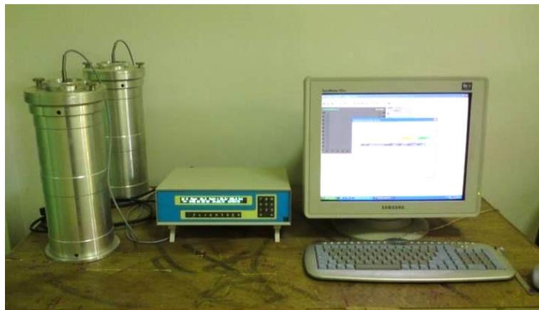
**Fig. 3 - Test setup for the hydration heat test.**
