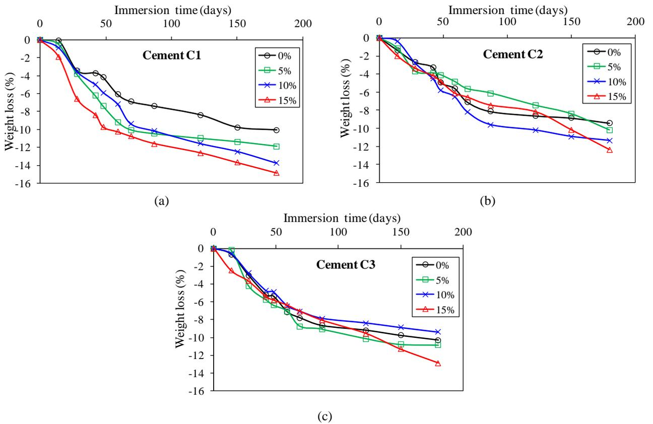
Fig. 10 - Evolution of weight loss mortars immersed in 3% H<sub>2</sub>SO<sub>4</sub>
