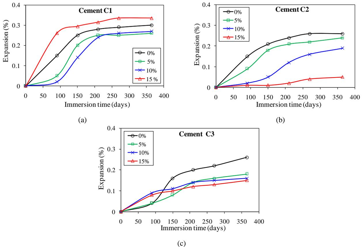
Fig. 7 - Evolution of expansion of mortars immersed in 5% Na<sub>2</sub>SO<sub>4</sub> solution.
