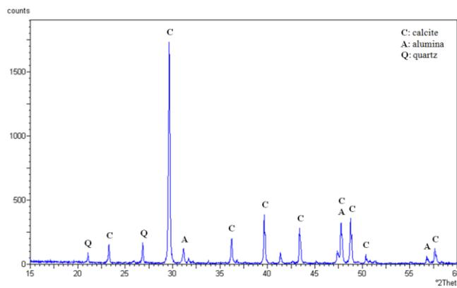
Fig. 2 - X-ray diffraction of limestone sand.
