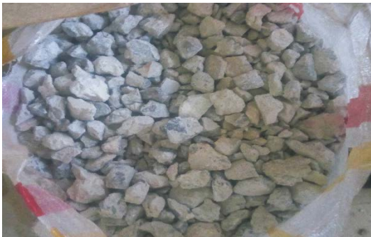
Fig. 3 - Recycled Coarse Aggregate (RCA)
