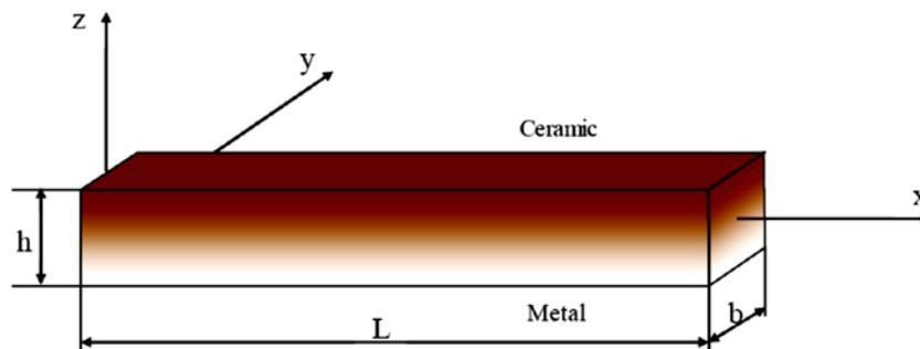
Figure1: Geometry and coordinates of the FG beam.
