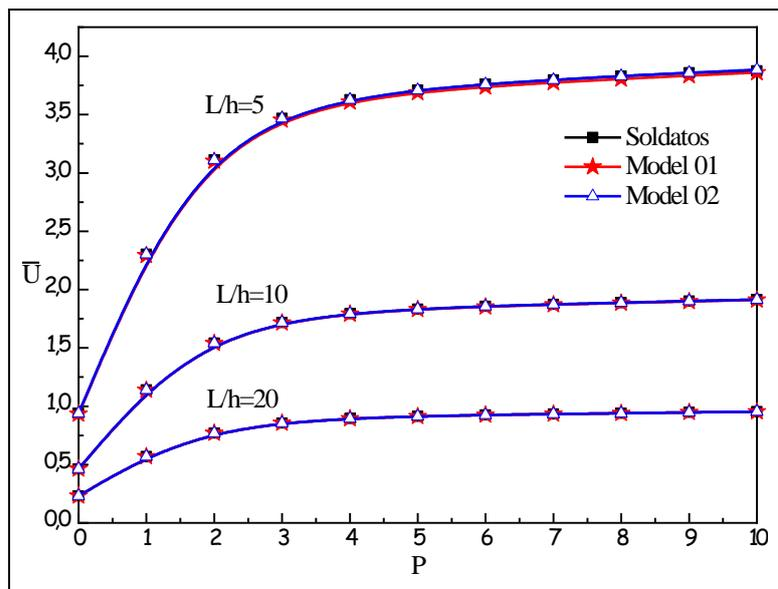
Figure 5: Variation of the non-dimensional axial displacement  $\bar{u}$  as a function of the power law index  $p$  for beams FG subjected to a uniform load with different  $L/h$  ratio.
