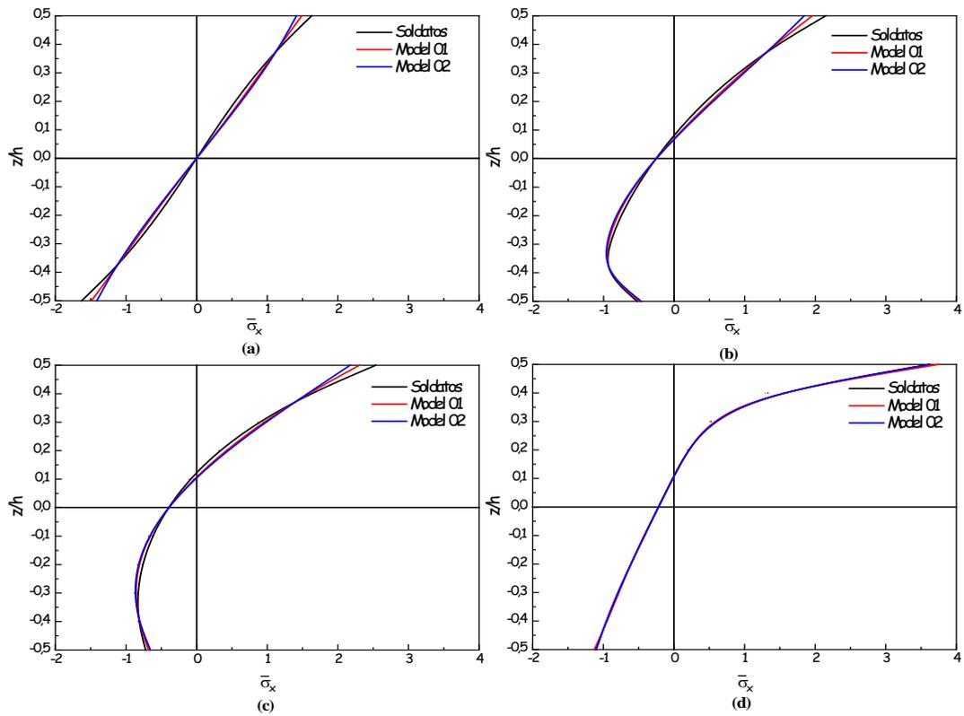
Figure 3: Dimensionless axial stress variation  $\bar{\sigma}_x(L/2, x)$  through the thickness of the FGM beam under uniform load with  $(L=2h)$ . (a)  $P=0$ , (b)  $P=0.5$ , (c)  $P=1$  and (d)  $P=10$
