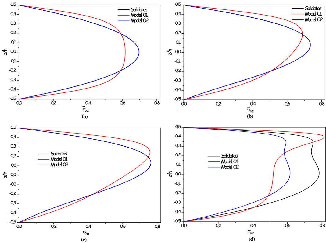
Figure 4: Dimensionless transverse shear stress variation  $\bar{\sigma}_{xz} (0, z)$  through the thickness of the FGM beam under uniform load with ( $L = 2h$ ). (a)  $P = 0$ , (b)  $P = 0.5$ , (c)  $P = 1$  and (d)  $P = 10$ .
