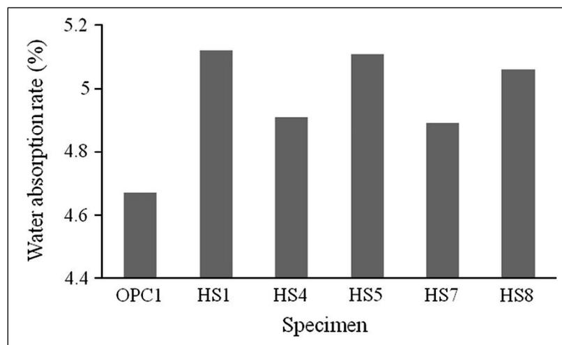
*Fig. 1- Water absorption rate of specimens [26]*
