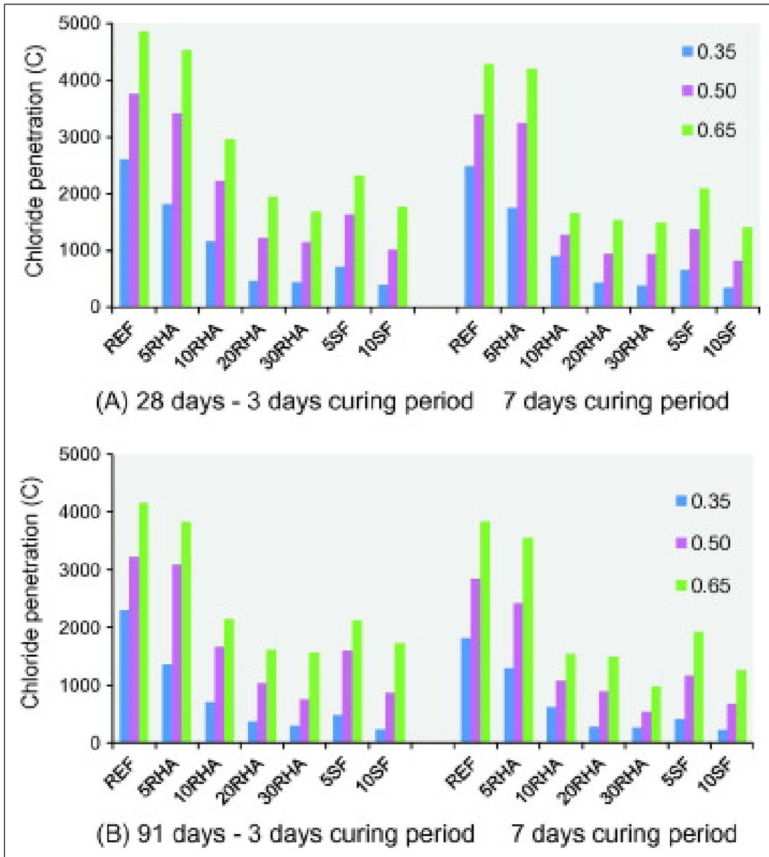
Fig. 4- Chloride penetration results [37]
