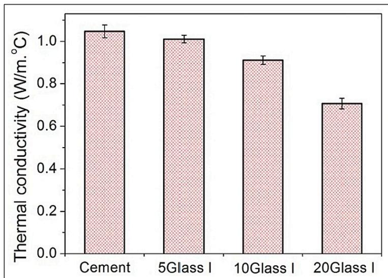
Fig. 6- Thermal conductivity of pastes [73]
