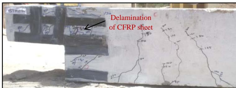
Fig. 17- Cracks Patterns for Strengthening beams NSTR2-A
