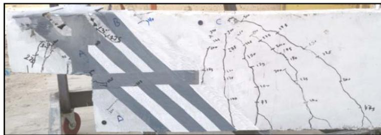
**Fig. 13- Cracks Patterns for Strengthening of beam HSTR1-B**
