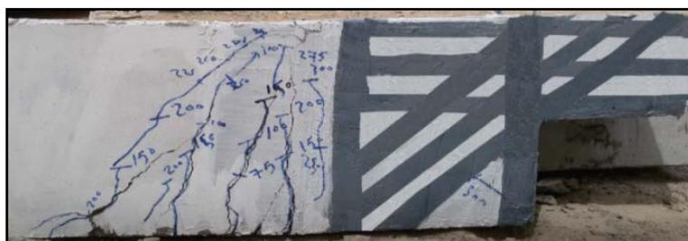
Fig. 20- Crack Patterns for Strengthening beams NSTR2-B
