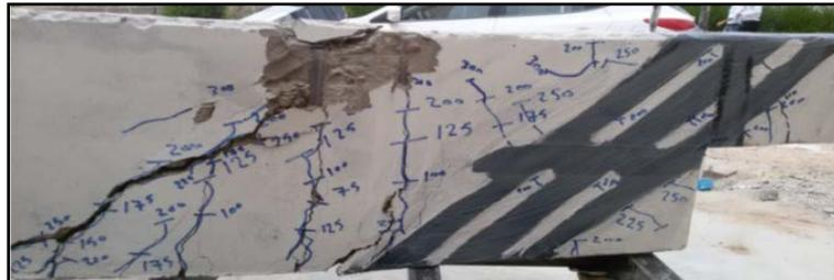
**Fig. 10- Cracks Pattern for the Specimen HSTR1-A**
