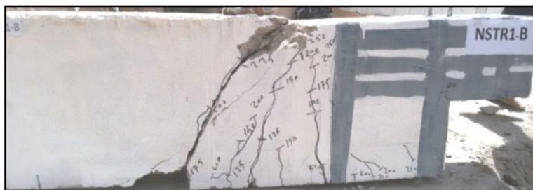
Fig. 19- Crack Patterns for Strengthening beams NSTR1-B
