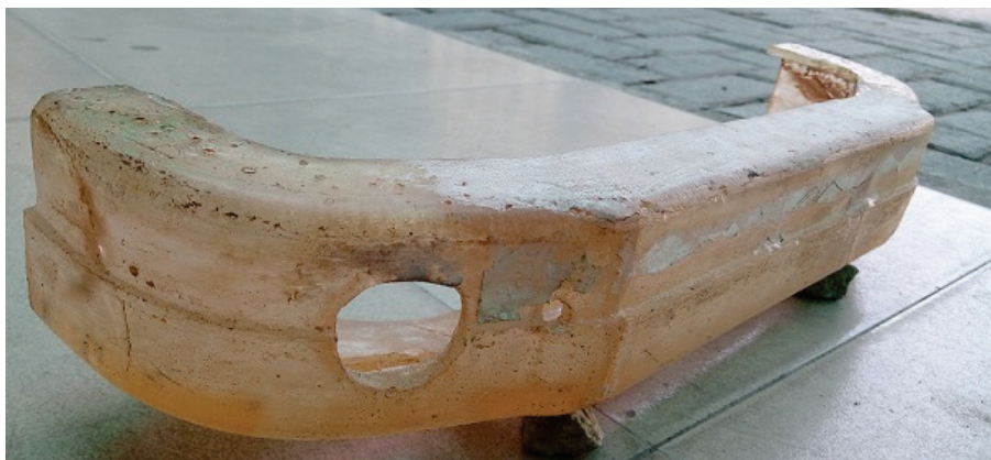
Fig. 17: Fabricated Epoxy-E Glass composite bumper prototype
