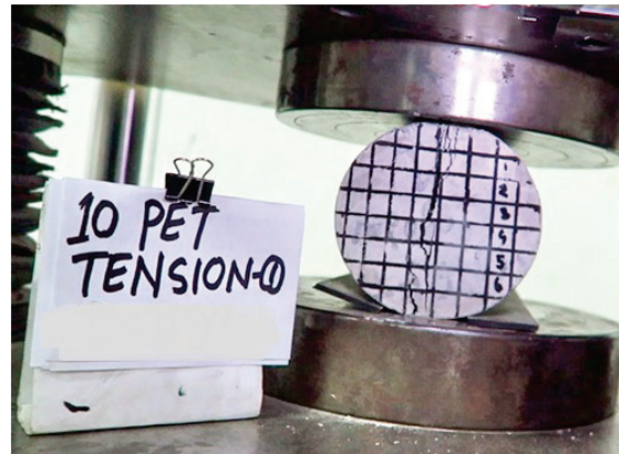
(d) Test specimens during splitting tension test
