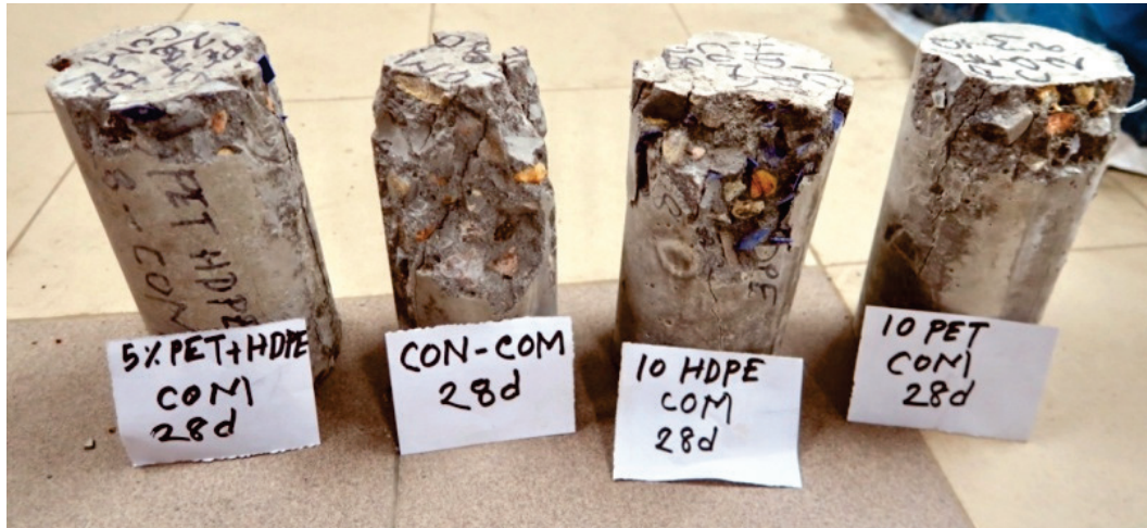
Fig.5 - Failure pattern of concrete specimens after compression test
