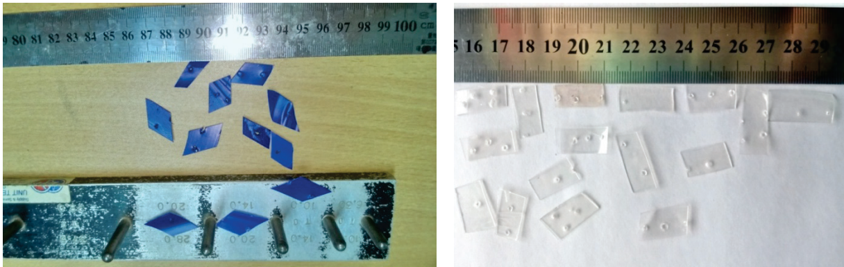
Fig. 3- Size measurement of HDPE and PET plastic by length gauge and scale
