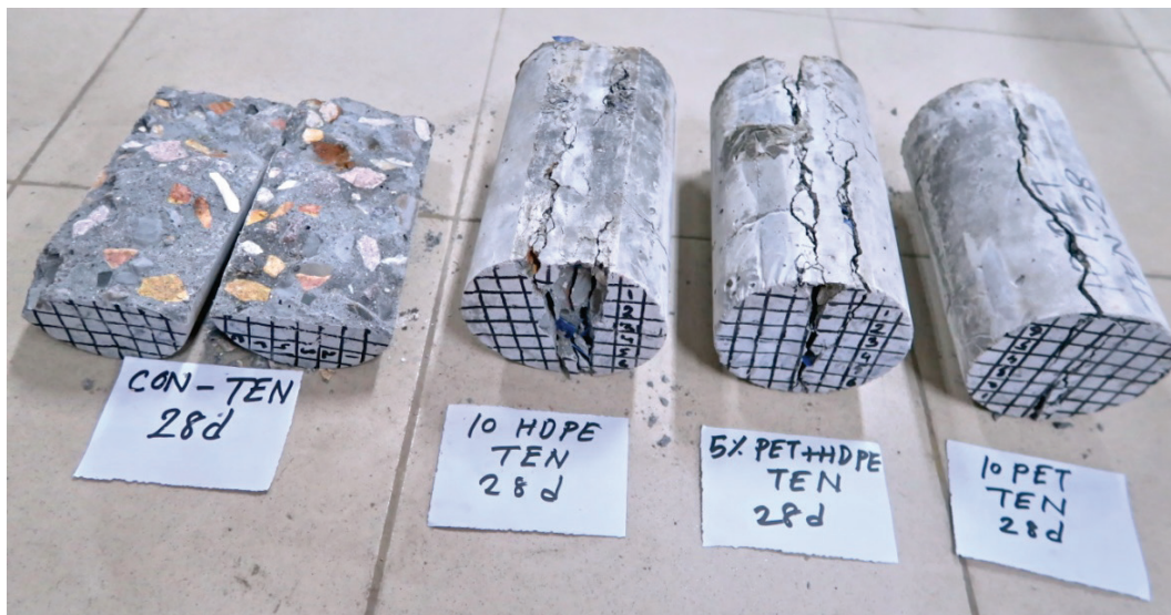
Fig.6 - Failure pattern of concrete specimens after splitting tension test
