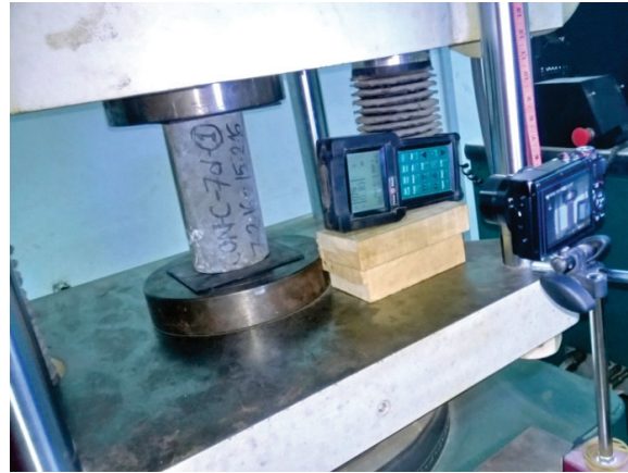
(b) Test setup of compression test
