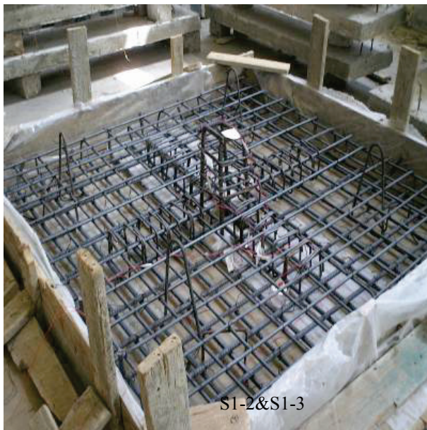
Fig.1 - Fabrication of the test specimens with stirrups shear reinforcement
