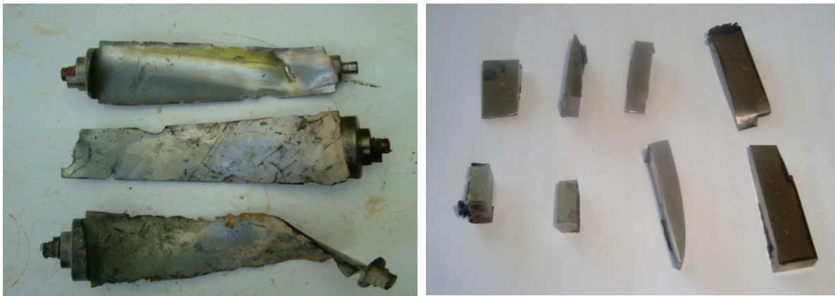
Fig.8-Turbine blades damaged samples.
