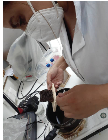
Figure 5 : Piece of builted comb of a known initial weight bonded inside the hoarding cage (original).
