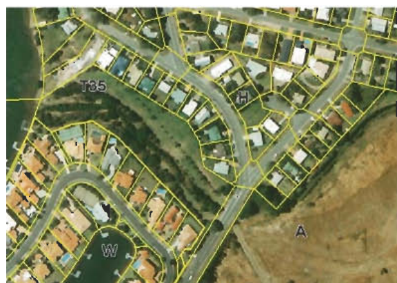
Fig. 4 Parcel-based classification of land cover including the percentage of tree cover. 'A' denotes 'Agriculture', 'H' – 'House', 'T35' – 35% of 'tree' cover, and 'W' – 'water'.
