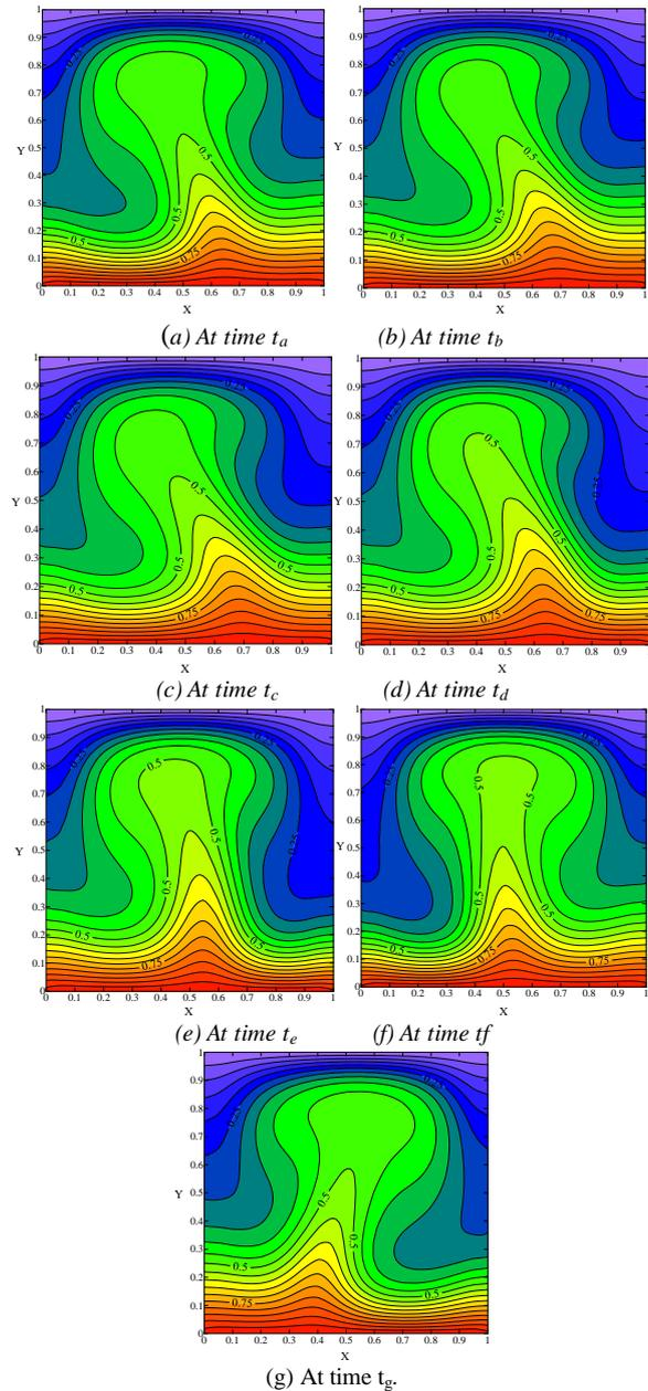
Figure 9. Isotherm line over time in one period of time for  $Ra_{c2} = 4.58 \times 10^4$ .
