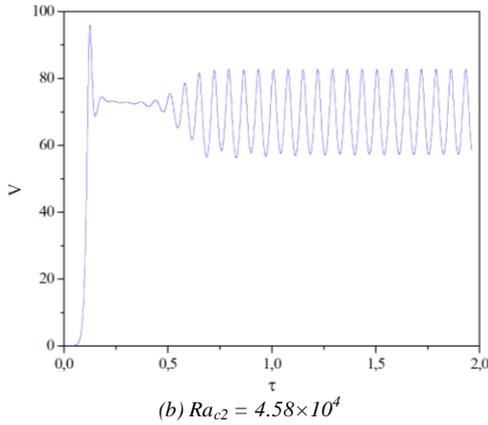
Figure 3. Time-dependent of dimensionless vertical velocity at the probe  $P_1$  for two value of Rayleigh number.
