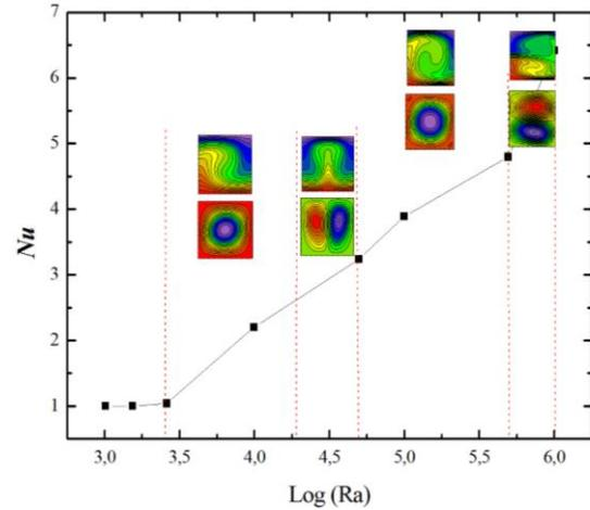
Figure 10. Logarithmic bifurcation diagram of Rayleigh-Bénard convection. The figure also summarizes Stream lines and isothermal line.
