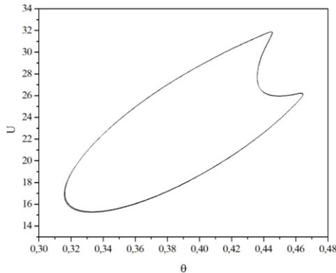
Figure 5. Phase portrait of horizontal velocity component in function of temperature at point  $P_2$  ( chosed arbitrary), for  $Ra_{c2} = 4, 58 \times 10^4$ .
