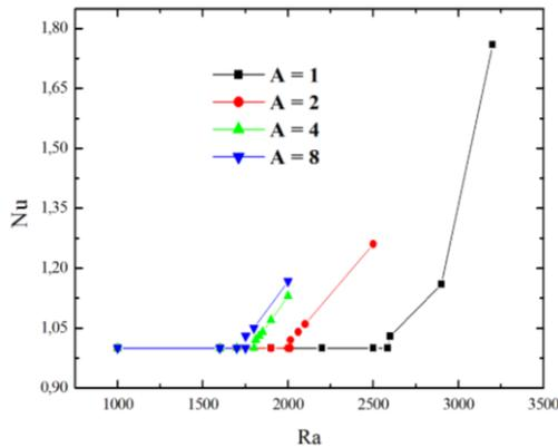
Figure 2. Average Nusselt Number in function of Rayleigh number for aspect ratio  $A = 1, 2, 4$  and  $8$ .
