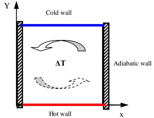
Figure 1. Schematic configuration of Rayleigh-Bénard probleme.
