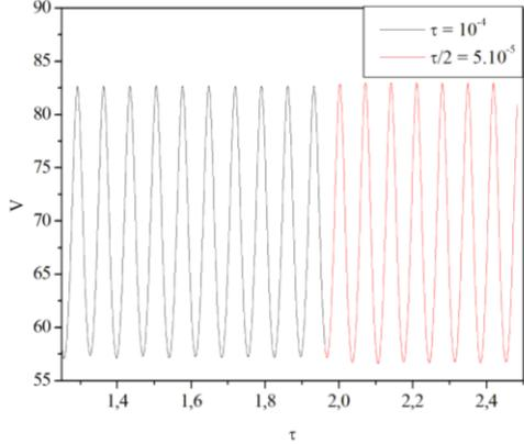
Figure 4. Time dependent of vertical velocity component for two time setp in  $P_1$  (chosed arbitrary) and for  $Ra_{c2} = 4, 58 \times 10^4$
