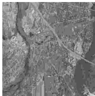
Figure 17. Reconstructed concord-aerial image for TCM/STBC, \text{bpp} = 0.5 , E_b/N_0 = 11 dB, \text{PSNR} = 21.58 dB
