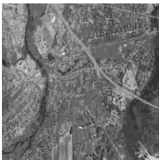
Figure 16. Reconstructed concord-aerial image for TCM-UGM/STBC, \text{bpp} = 0.5 , E_b/N_0 = 11 dB, \text{PSNR} = 22.26 dB
