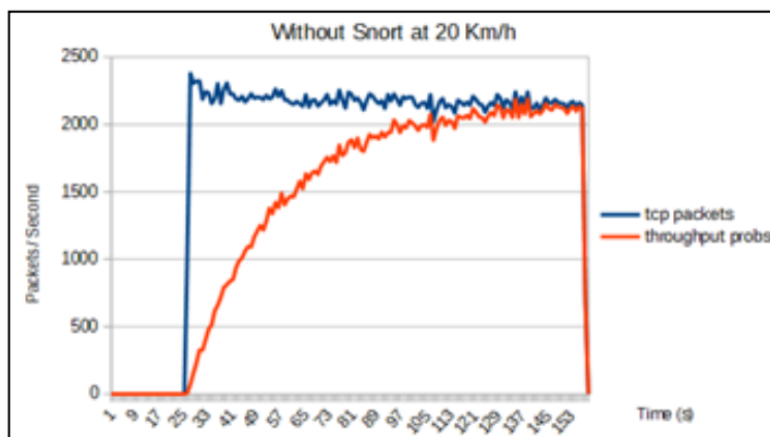
Fig. 4. The impact of the DoS attack on the target machine at 20 Km/h
