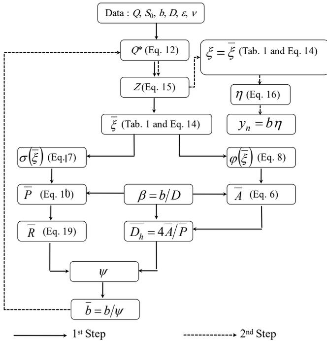
Figure 3: Flow chart for normal depth calculation
