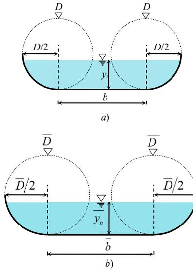
**Figure 1: Schematic representation of the considered channels. a) Current channel; b) Referential rough model**
