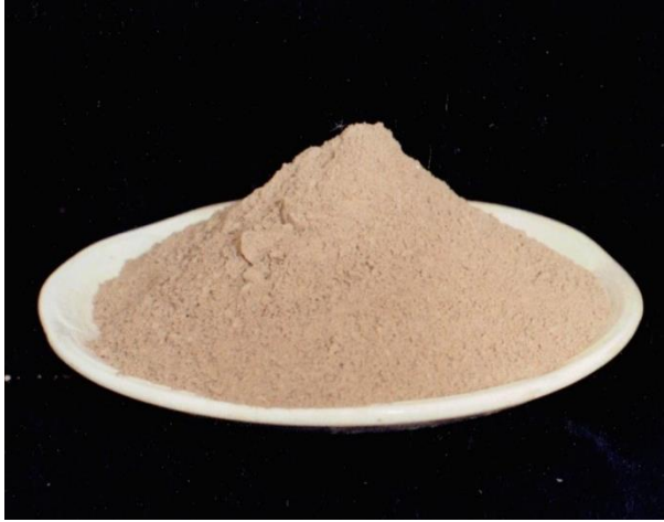
Figure 23: Dust obtained after drying and grinding of the mud (Initial dust) (Photo Remini, 2016)
