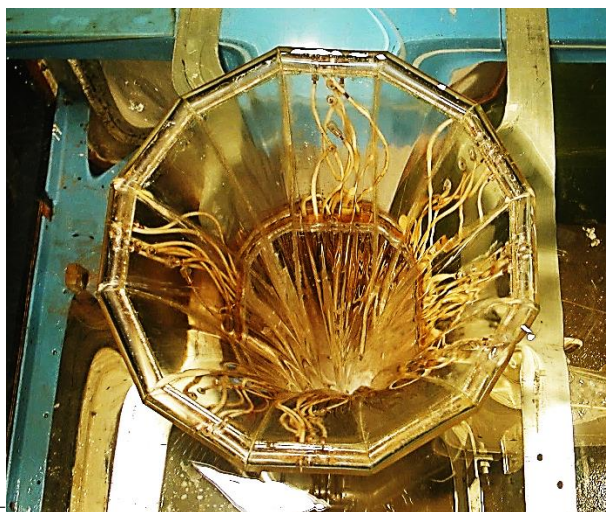
Figure 8: photo internal cavity model water inlet funnel with polyethylene hoses.
