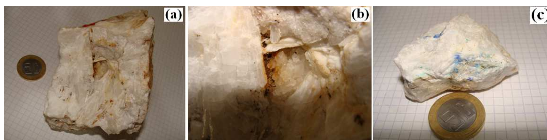
Fig.2: The photomicrograph of the barite samples; inlaid barite, \text{SiO}_2 (a, b), and blue spot known as the azurite mineral (c).
