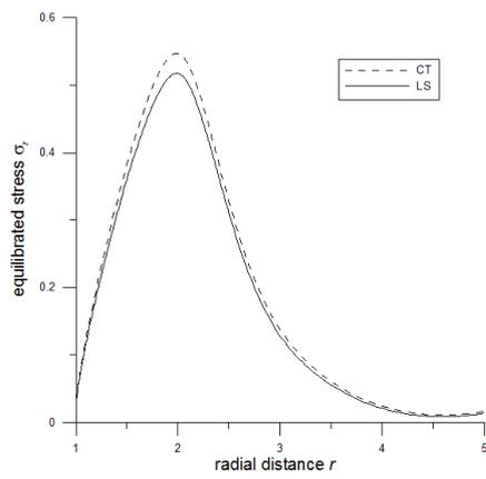
Fig. 2 – Variation of equilibrated stress  $\sigma_r$  w.r.t. radial distance  $r$ .
