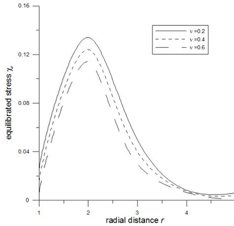
**Fig. 7** – Variation of equilibrated stress  $\chi_r$  w.r.t. radial  $r$ .
