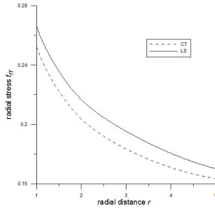
Fig. 1 – Variation of radial stress  $t_{rr}$  w.r.t. radial radial distance  $r$ .
