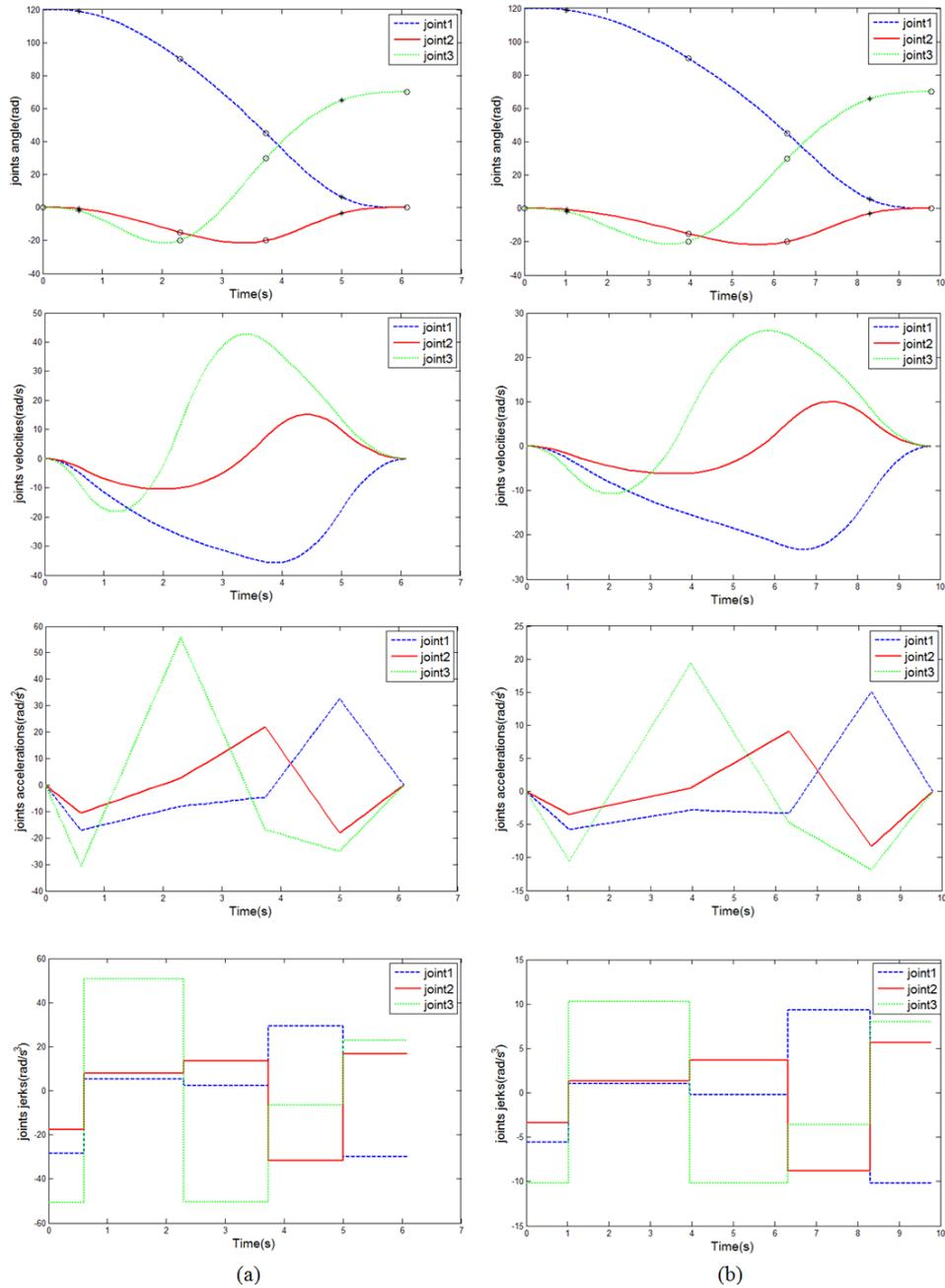
**Fig. 2** – The results of the simulation showing the trajectories of each joints angles (the circles indicate the knot positions and the crosses indicate the two dummy knots), velocities, accelerations and jerks of the glass substrate handling robot (a) :  $K_J / K_T = 0.02$  and (b) :  $K_J / K_T = 0.03$
