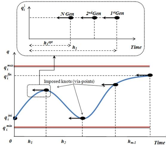
**Fig. 1** – Representation of the Cubic Spline Trajectory with the horizontal movement of the intermediate knots and the end point after generation.
